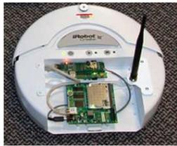
Figure 1: An iRobot Create and its wireless card.
