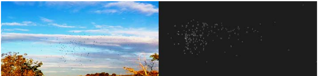
Figure 3: Mask created by applying the GMG algorithm on the bird video feed. Left: the real video feed where the black dots are the birds in the frame. Right: the background subtraction mask created by GMG where the white dots represent the birds.
