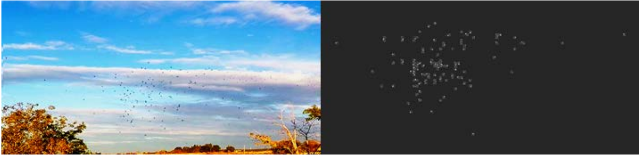
Figure 2: Mask created by applying the MOG algorithm on the bird video feed. Left: the actual video feed and the black dots are the birds in the frame. Right: the background subtraction mask created by the algorithm; the white pixelated dots represent the birds separated from the background.
