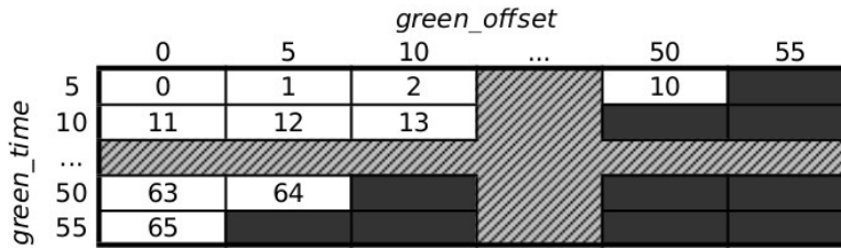
Figure 3. The signal scheme index for each DCEE agent, and its corresponding ( green_{offset} , green_{time} ) value, defining an active phase of 60s. Note that green_{offset} and green_{time} increase at five-second intervals, a necessary discretization.
