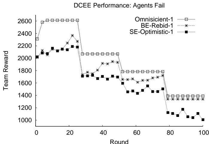
**Fig. 22:** This graph shows how agents can automatically recover after a failure of 2 agents after every 25 rounds.
