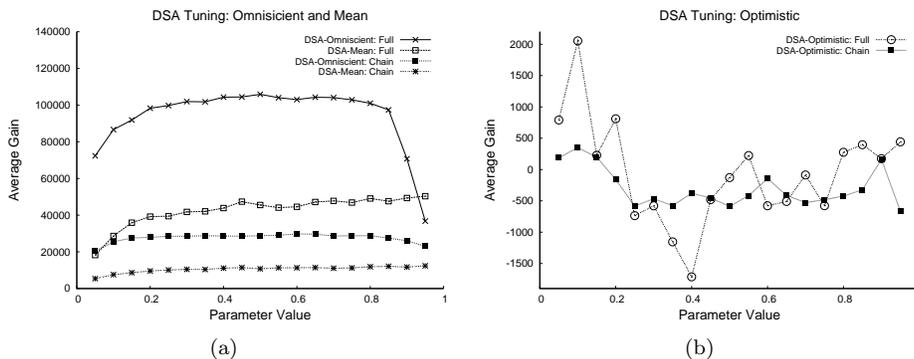
Fig. 24: Tuning the value of  $p$ , the parameter controlling the behavior of DSA, can be difficult. For instance, in (a), a mid-range value of  $p$  maximizes the performance of the DSA-Omniscient algorithms, while the highest value of  $p$  maximizes the performance of DSA-Mean. (b) suggests that there is little regularity to the performance of DSA-Optimistic with respect to the value of  $p$ .
