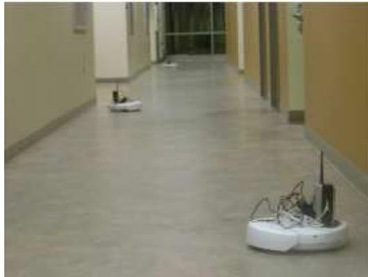
**Fig. 3:** Three iRobot Creates with on-board computers
