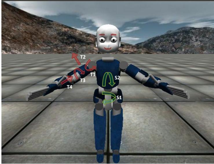
**Figure 7.** iCub joints controlled in the source task (green arrows) and the target task (red arrows), where each joint corresponds to a state variable. The arrow head shows the positive direction of the joint (+) and also represents the positive action on that joint (e.g., S1+.)
